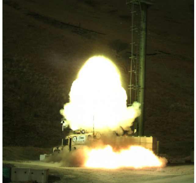
Figure 18: Testing of Falcon's Linear Rocket Motor on a mock-up of an armoured Land Rover driving over an improvised explosive device. The top plume is from the Linear Rocket motor and the bottom plume is from the improvised explosive device.
