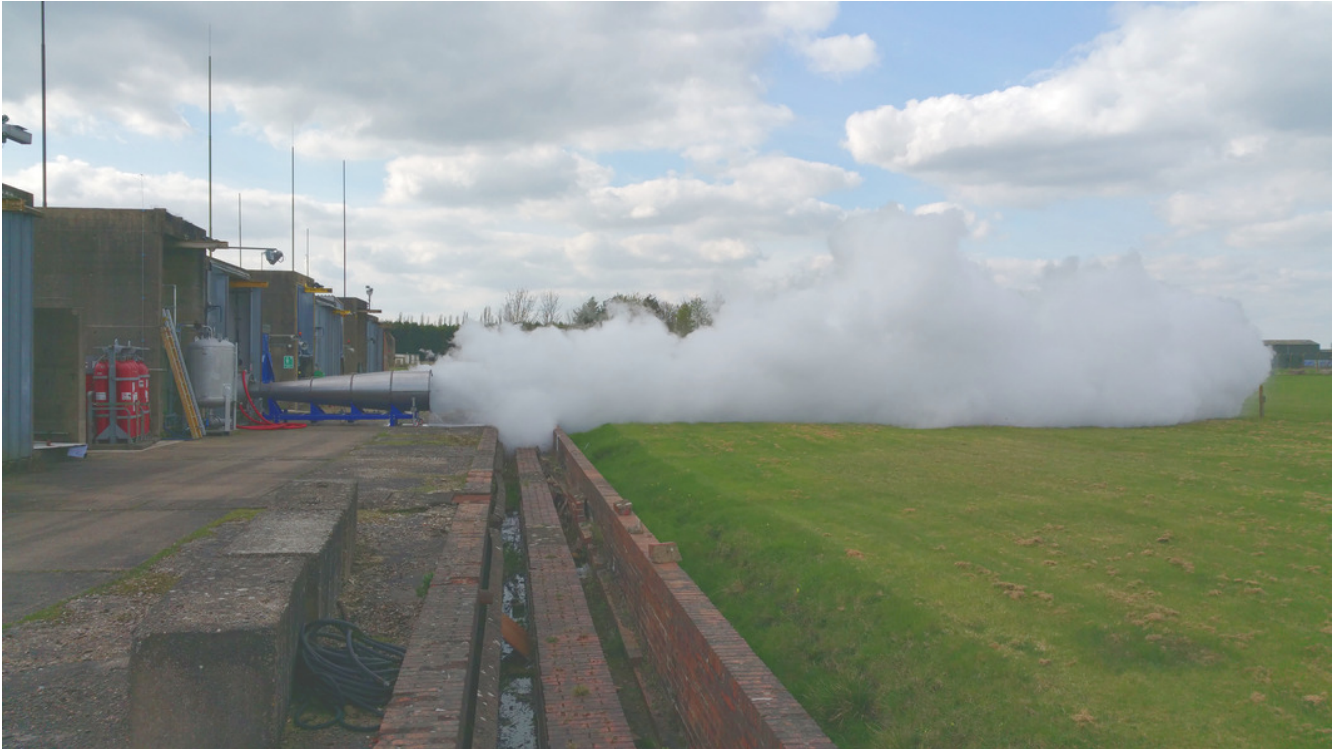
Figure 5: Sound suppression testing at AEL's J2 test facility. A custom water spray system and diffuser duct cools and slows the plume to significantly reduce the emitted sound.
