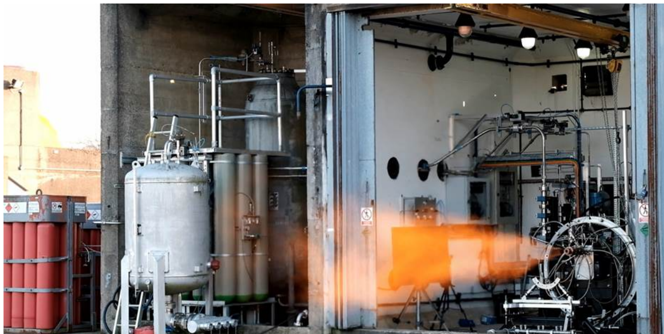
Figure 7: Hydrogen rich gaseous injector testing, to validate the performance of a novel H 2 /O 2 injector for inlet to a turbopump.
