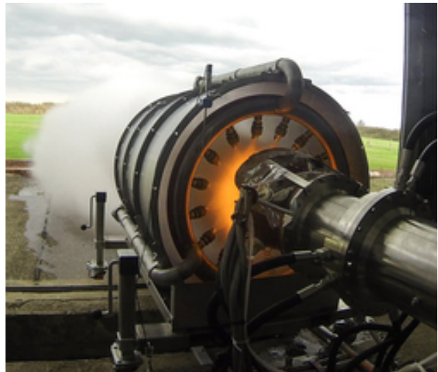
Figure 6: Water spray injection into the plume of the 20kN STOIC engine for sound suppression testing.
