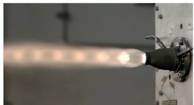
Figure 11: Ignition sequence for LEROS 4 undergoing early development testing at the Westcott J3 sea-level facility.
