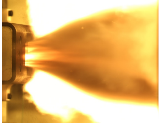
Figure 17: Fast burning propellant testing for Falcon's Linear Rocket Motor on the Falcon 1MN test stand at Westcott.
